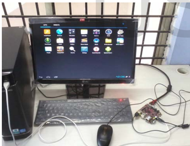
Fig. 2: Overall hardware connections to BeagleBoard XM To develop android application for Smart TV system, Software requirements are,
